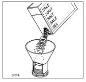
The salt container will require topping up periodically. You are reminded of this by the salt indicator light on the control panel which comes on when the salt has finished.
